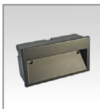
EMEX0199 EX0125REW EMBUTIDO 200x106 mm LED 9.6W DC700mA 179LM 3000K IP65 193x99mm
